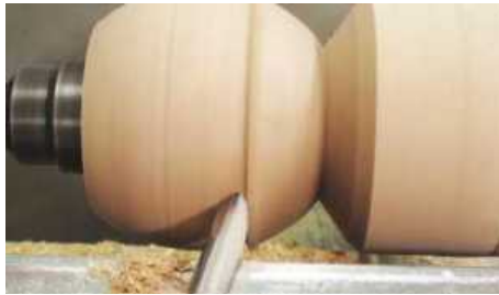
▲ Pic.2 Make 'V' cuts on the marks and round over the three beads for the body. Start with the handle low and lift as you work through the cut
